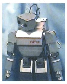
objects based on features such as bright colors and sharp edges. Then the robot uses a speech synthesizer to say out loud what the instructor is looking at.
